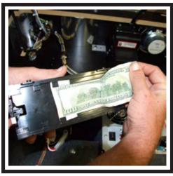
**Step 3**Remove Bills, then refit the stacker to the BV50 with an upwards click to locate.
