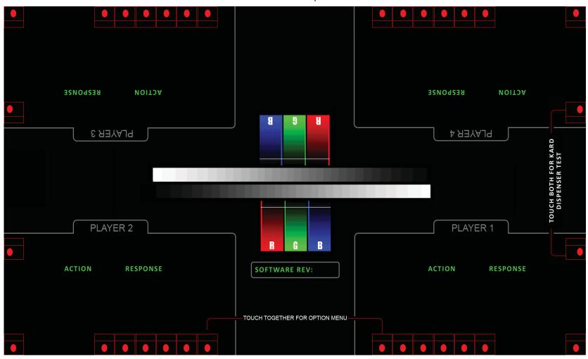
Touch screen buttons together to test Card vending. (vends only 1 card per entry into test screen)
