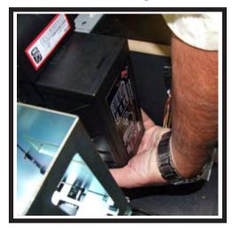
**Step 1**Hold Stacker and place a finger on the latch button located on the base of the BV50 and gently slide the button.
