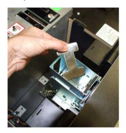
Reach into dispenser and remove the 'H' shaped weight as shown
