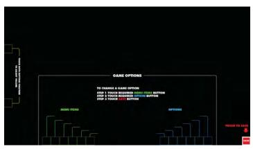
You enter the option screen via the test screen. Follow on screen instructions to change options, then touch the Save button to save and exit.
