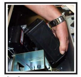
**Step 2**Press the Stacker down and lift clear of the bill acceptor.
