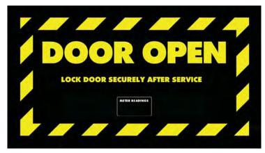
This screen is a security screen and shows meter readings. It is displayed whenever the top door is opened
